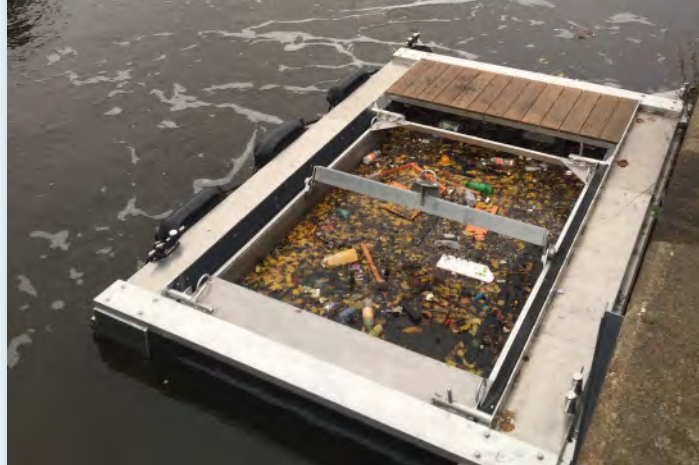
A Bubble Barrier installation collects plastic trash in Amsterdam. Photo courtesy of The Great Bubble Barrier.
