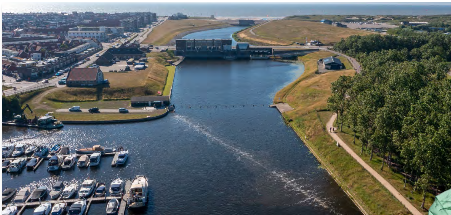
An aerial view shows the diagonal Bubble Barrier in Katwijk, Netherlands, that guides trash into a catchment area for removal but does not block watercraft or wildlife. Photo courtesy of The Great Bubble Barrier.
